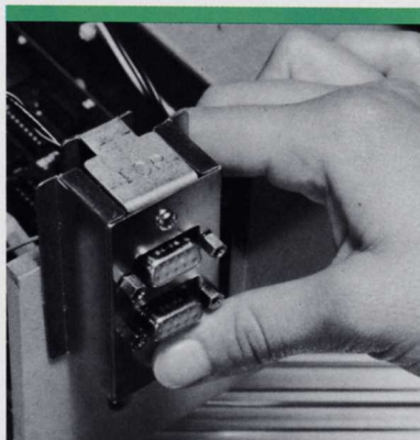
Figure 23. Slide assembled clamp into notch in back panel.
