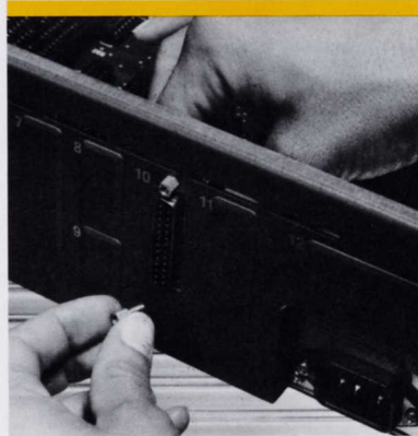
Figure 41. Insert and tighten screws.
