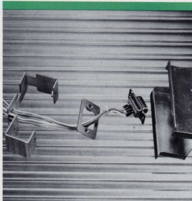
Figure 20. Thread cable and connector through nut plate and opening in clamp.
