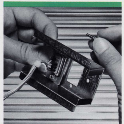
Figure 21. Attach connector to clamp using the screws and nut plate.
