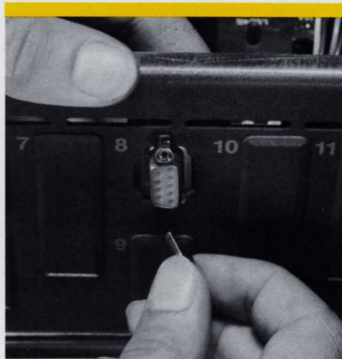
Figure 17. Insert and tighten screws.
