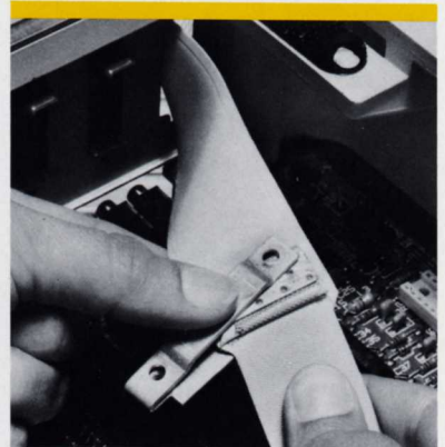
Figure 5. Slide cable and flap into clamp.
